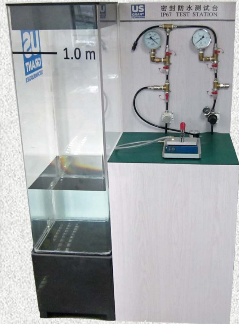
Water submersion testing station – vacuum & pressure
